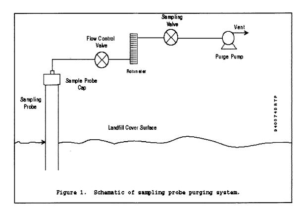
4.4 Sampling Procedure. Open the sampling valve and use the purge pump and the flow control valve to evacuate at least two sample probe volumes from the system at a flow rate of 500 ml/min or less (30.5±3.1 m³/min). Close the sampling valve and replace the purge pump with the sample tank apparatus as shown in figure 2. Open the sampling valve and the sample tank valves
