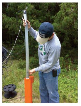
Lower Loup Natural Resources District staff utilizing a passive diffusion sampler to sample a monitoring well near Duncan, NE.
