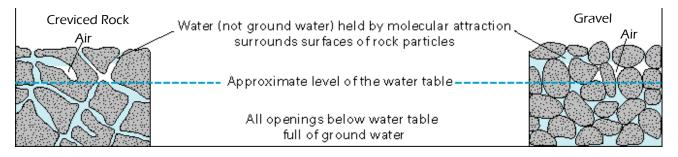
Figure 1. Basic aquifer concepts (U.S. Geological Survey).
