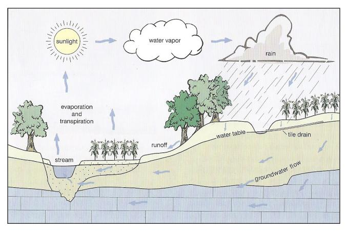
Figure 2. Generalized hydrologic cycle. (Prior, 2003).
